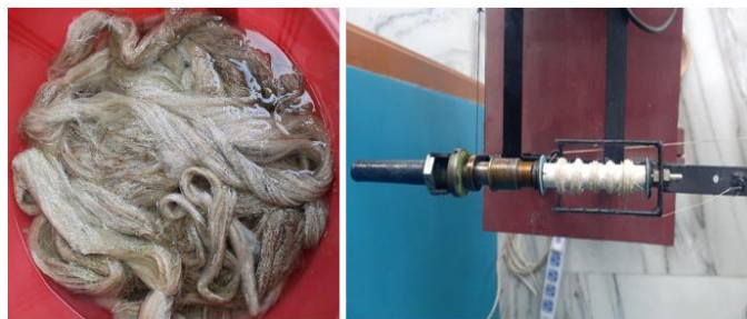
Fig. 2 Pictorial view of pineapple leaf fiber and prepared pineapple yarn
