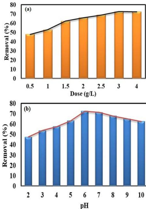
Fig. 4. Effect of mBC-400 dose (a) and pH (b) on removal of As (III)
