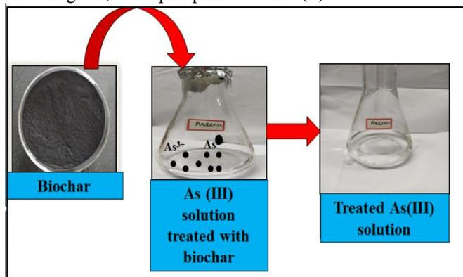
Fig. 2. Pictorial representation of treatment of As(III) solution with biochar (mBC-400)
