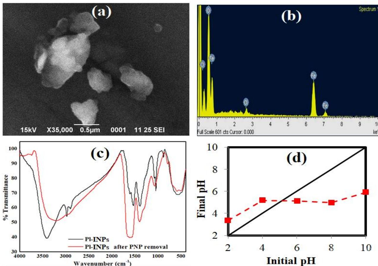
Fig. 1 a) SEM analysis, b) EDS, c) FTIR and d)  $pH_{ZPC}$  analysis of PI-INPs
