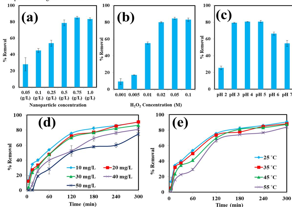
Fig. 2 a) Optimization of Nanoparticle concentration, b) optimization of  $\text{H}_2\text{O}_2$  concentration, c) optimization of pH, d) optimization of PNP concentration and e) optimization of temperature.
