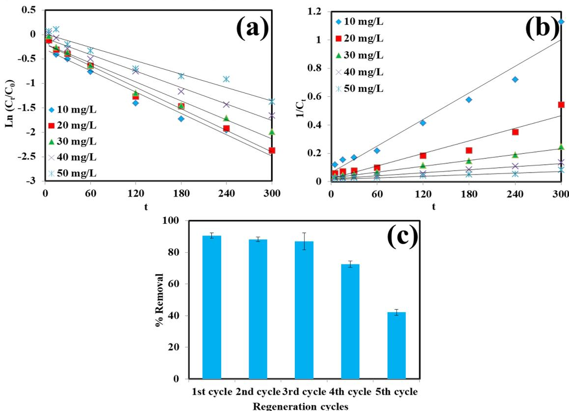
Fig. 3 a) Pseudo-first-order kinetic plots, b) pseudo-second-order kinetic plots for PNP degradation and c) Regeneration of PI-INPs
